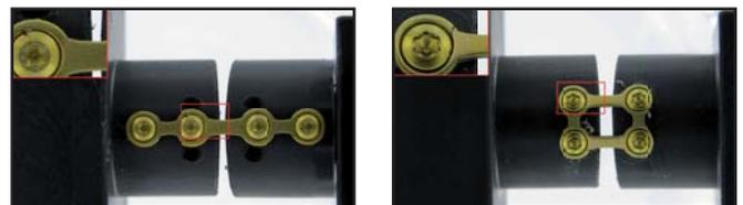
Figure 8 Non-locking plates after testing. Left: A-4300.01 (buckled), right: 4300.51 (fractured)
