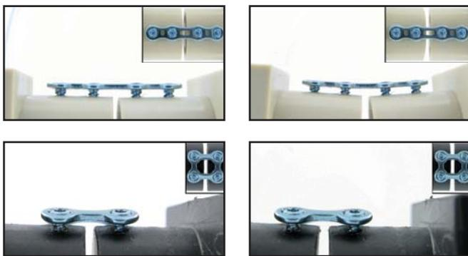
Figure 7 TriLock 1.5 plates before (left) and after (right) testing. Top: A-4350.01, bottom: A-4350.50
