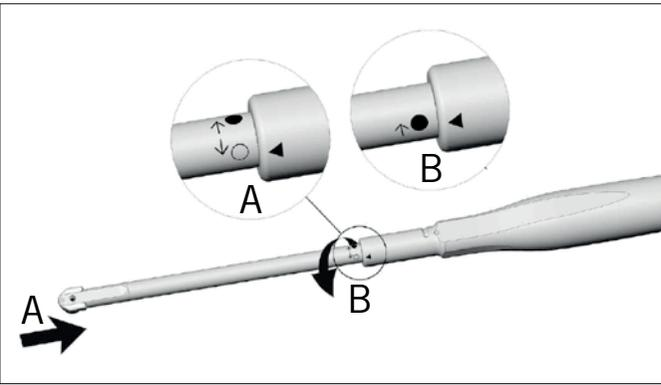
**A** Insert the head into the sheath until it engages
