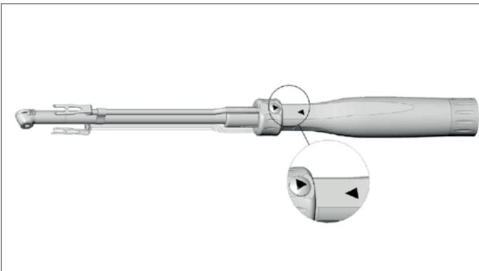
Turn the screwholding fork into the unlocking position
