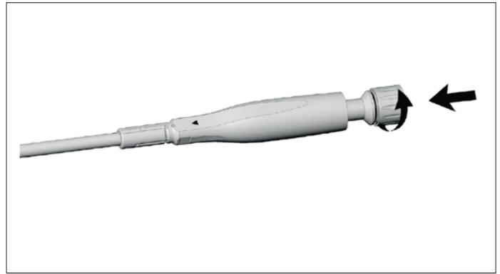
Push the shaft into the sheath and screw this tightly in place
