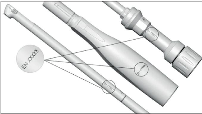
Check that the EN number on the sheath, head and shaft match
