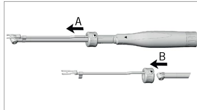
**A** Push the screwholding fork forwards until the clip releases
