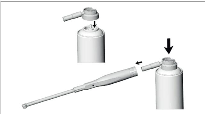
Oil service – After internal cleaning, before each sterilization
