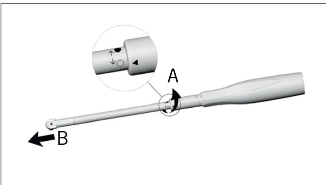
**A** Loosen the head from the sheath by turning it from «●» to «○»
