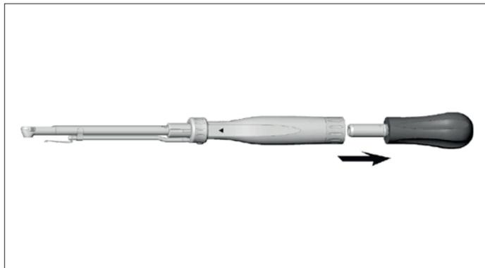
Remove the screwdriver's rotation knob
