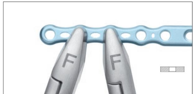
When bending the flap of the posterolateral plate, the plate bending pliers with pins must be held so that the letters «F – FLAT PLATE THIS SIDE UP» are legible from above. This ensures that the plate holes are not damaged.
