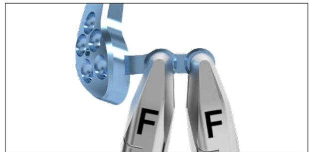
While bending, the plate must always be held at two adjacent holes to prevent contour deformation of the intermediate plate hole.
