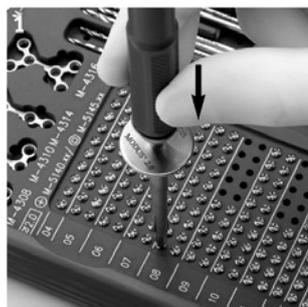
1. Position the screwdriver directly in line with the screw.
