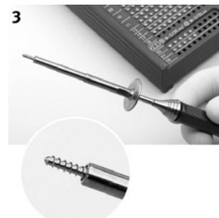
3. The screw is held securely by the tension sleeve.
